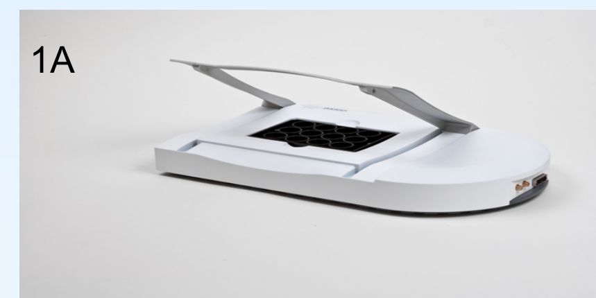
Figure 1A: The Maestro – Axion BioSystems • 768 stimulating and recording channels • SBS-Compliant Multiwell MEA plates • Accommodates 12, 48 and 96 wells • Fully integrated heater with software controls • Automated electrode characterization & diagnostics
