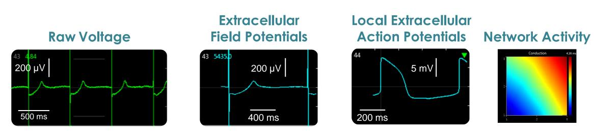
Raw voltage signals are processed in real-time to obtain extracellular field potentials from across the network, providing a valuable electrophysiological phenotype for applications in drug discovery, toxicological and safety screening, disease models, and stem cell characterization
