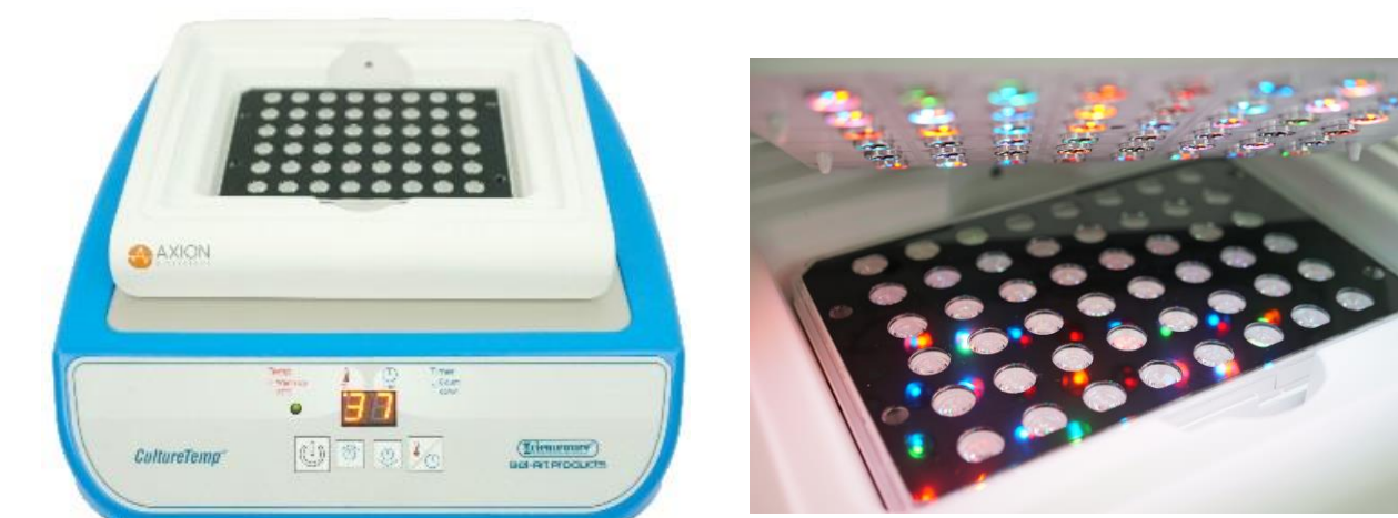
Dissociated DRGs were cultured on OptiClear 48 plates and stimulated with the Lumos device. The Lumos Ecbase was used to maintain environmental control during stimulation.
