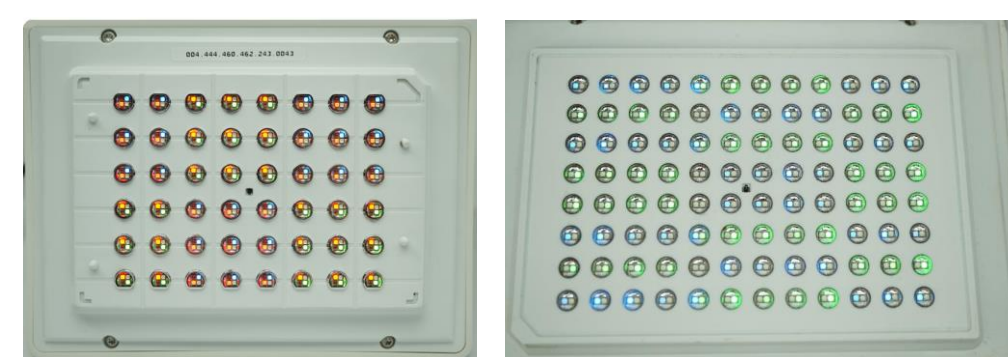
Swappable head units for 24-, 48-, and 96-well plates
