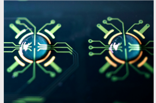
Base of the BioCircuit MEA 24 plate (M384-BIO-24) with the wells removed. On-plate spotting guides center the droplet over the recording electrode array, increasing plate preparation speed and accuracy.
