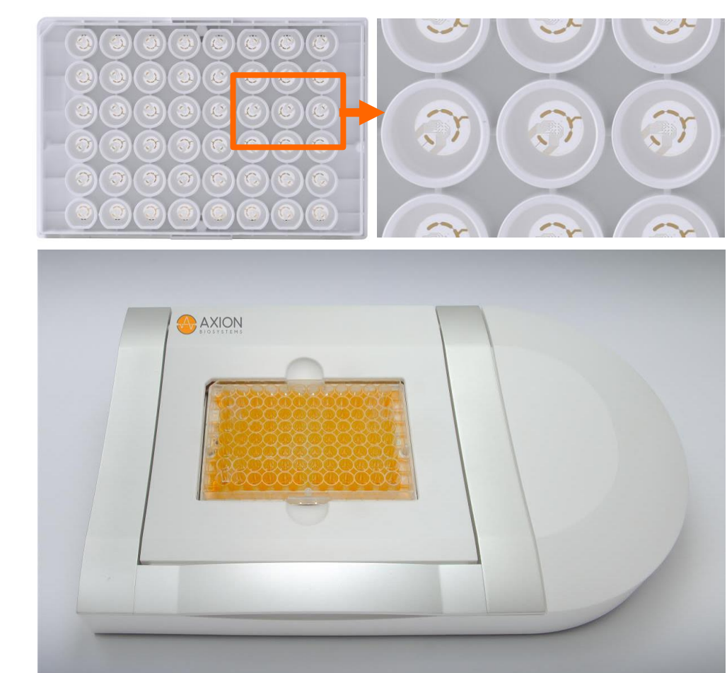
Axion's Maestro multiwell microelectrode array (MEA) platform enables functional cellular analysis on the benchtop with 768 electrodes across all plate formats.
